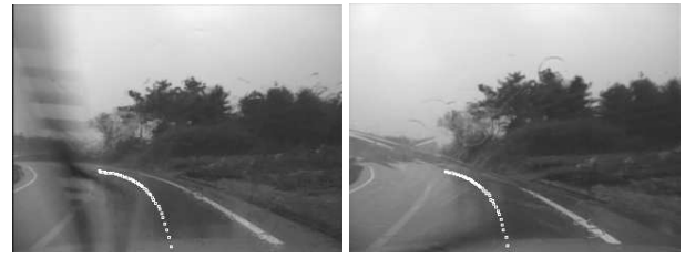
Figure 5: Motion is correctly estimated during moderately rainy condition. The windshield wipers and rain drops on the windshield are ignored by the robust algorithm.
