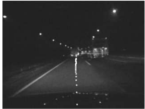
Figure 6: The markings on the road illuminated by the car headlights are sufficient for motion estimation.
