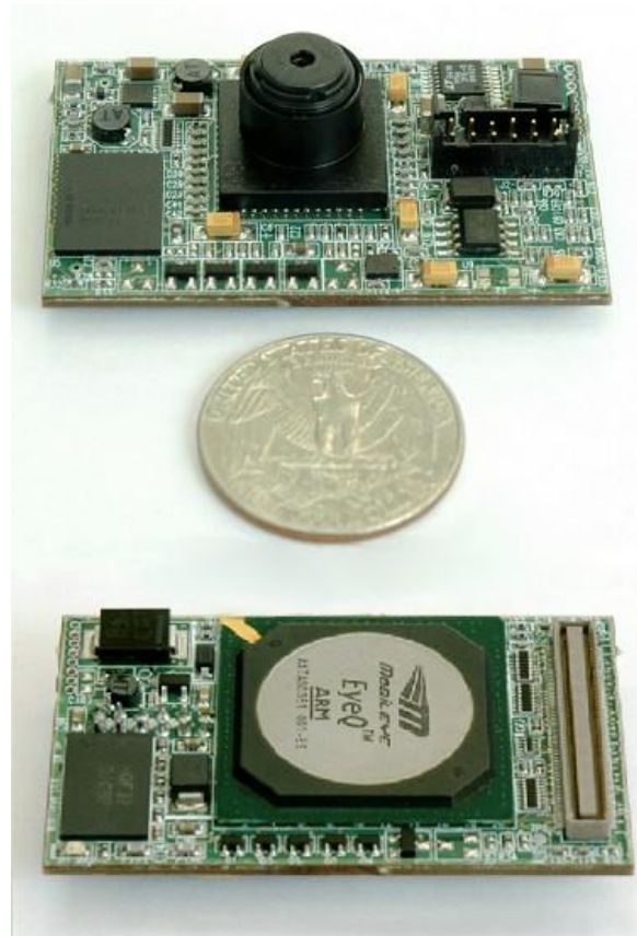
Figure 4. The SeeQ board measures only 53\text{mm} \times 33\text{mm} and is an example of a compact embedded application which includes processor, HDRC image sensor, memory and power supply.
